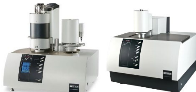
Figure 7. Thermal Analysis Instruments (a) NETZSCH STA 449 F3 Jupiter (b) NETZSCH LFA 457 HyperFlash
