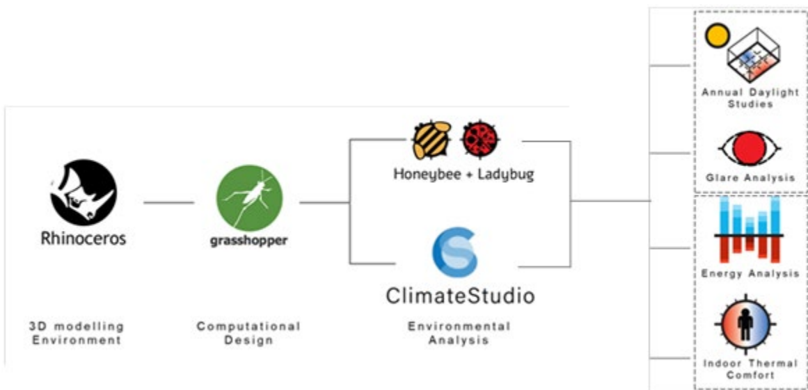
Figure 30: Flow chart demonstrating the interoperability between energy and daylighting plugins, and outputs from energy/thermal and daylighting analysis.
