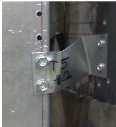
Figure 25 Failure modes of web clip angle reinforced CFS connections [23].
