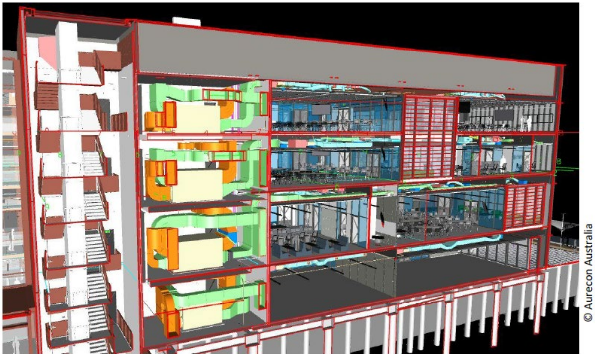
Figure 14. BIM model of the Woodside Building for Technology and Design's mechanical system
