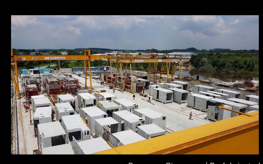
Dragages Singapore | Prefabricated Prefinished Volumetric Construction
