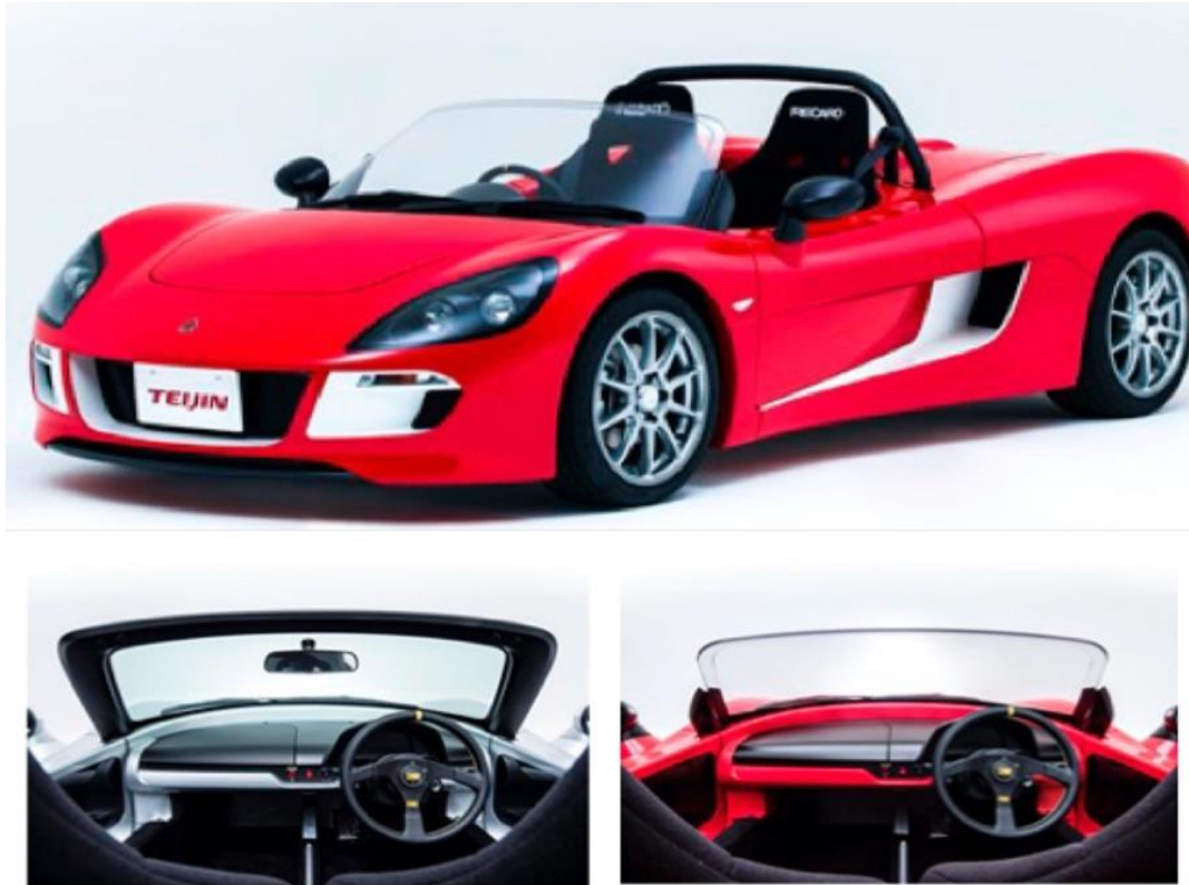
Figure 17. Tommykaira ZZ with Polycarbonate-resin pillar-less front window; conventional glass front window with an A-pillar (left) and a newly developed pillar-less front window (right).
