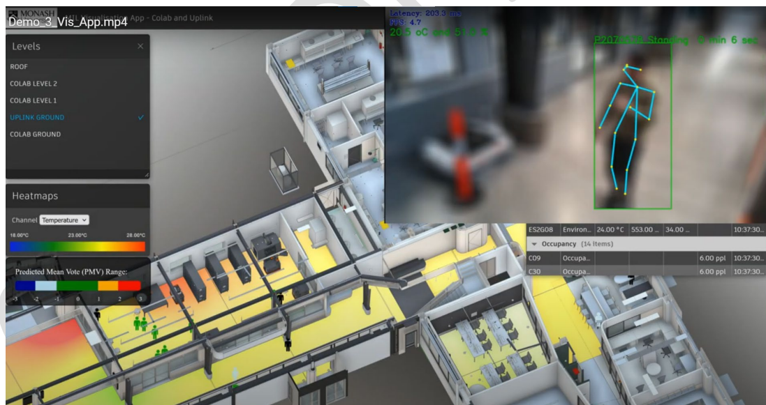
Figure 27. Real-time thermal comfort measurement and visualisation in MIL-DT
