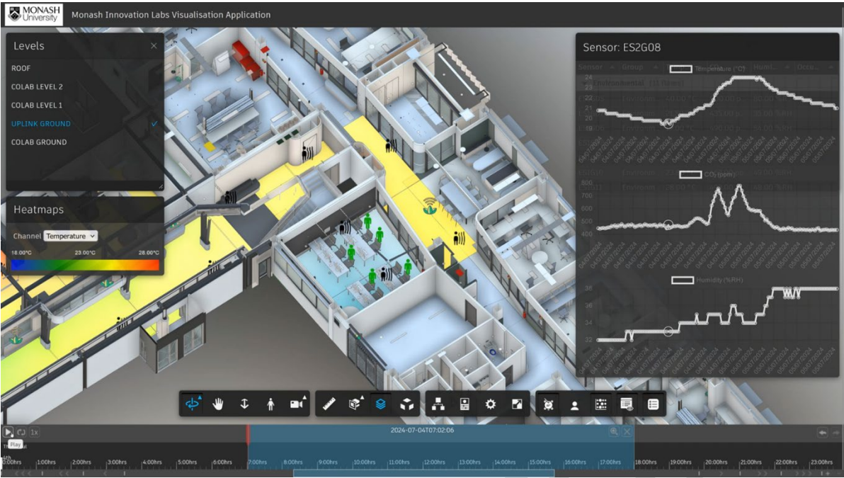
Figure 23. Real-time DT visualisation platform showing a temperature spatial heatmap and trendline plots
