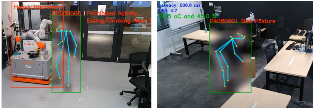
Figure 25. Computer vision-based detection of workplace safety and health risks (left: eating/drinking near a machine; right: bending the back when lifting heavy load)
