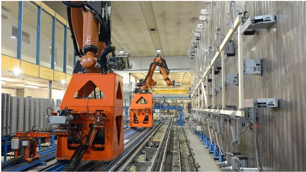
Figure 20 Trussmatic system – assembly
