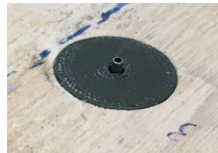
Figure 4. Wind Tunnel Model of D & T Building viewed from above, showing location of Irwin probes installed in the vicinity of the building (top); hot-film anemometer (centre); close-up image of Irwin probe.
