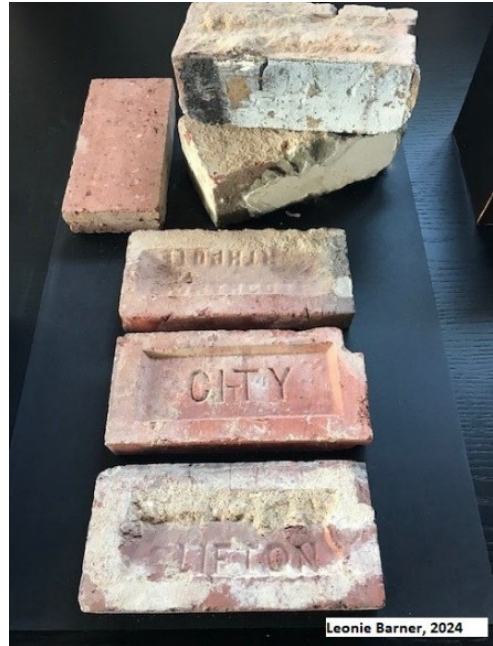
Examples of reuse: Pile of bricks waiting to be reused. Examples of bricks recovered from the building during the restoration. The brick in the upper left corner has been cut in half to be used as a pavement brick. Bricks are locally made.
