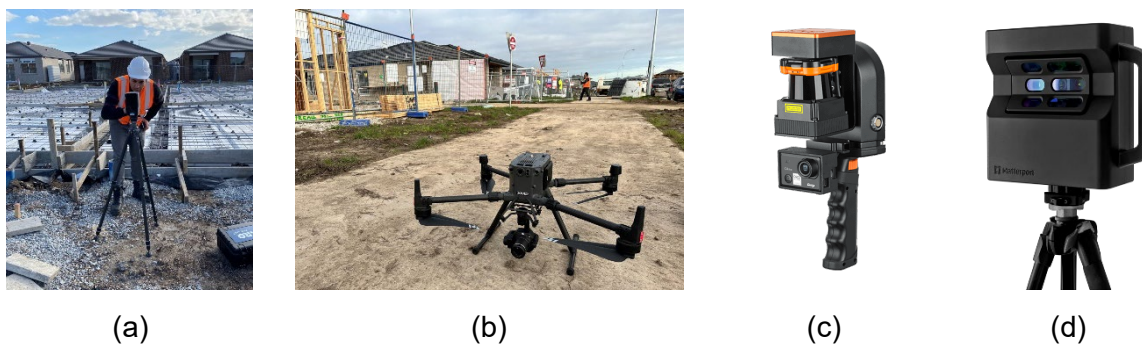
Figure 6.1: The four reality capture sensors used in the case study: (a) Faro Focus S TLS, (b) Emesent Hovermap ST, (c) Geoslam Zeb Revo, (d) Matterport Pro 2
