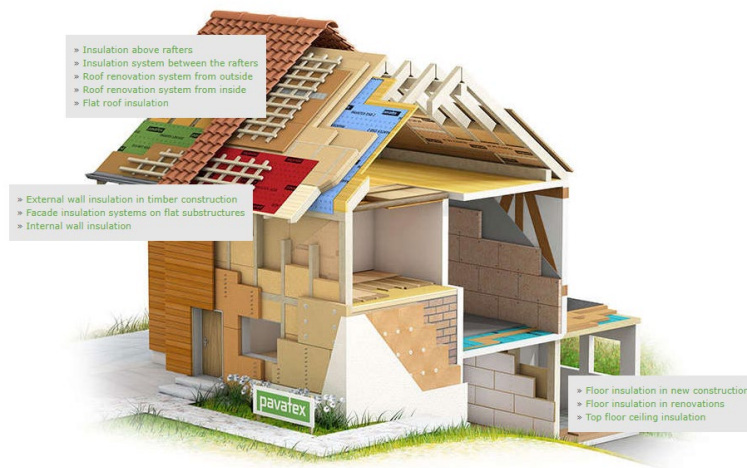
Figure 1 Typical insulation classes for timber fibre insulation (Pavatex – Switzerland (2021))
