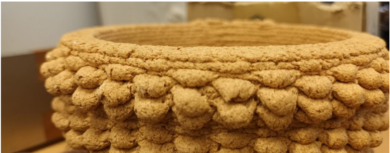
Figure 28. 3D-printed research, organic composite materials
