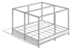
3d: Loft level steel frame supported by steel columns
