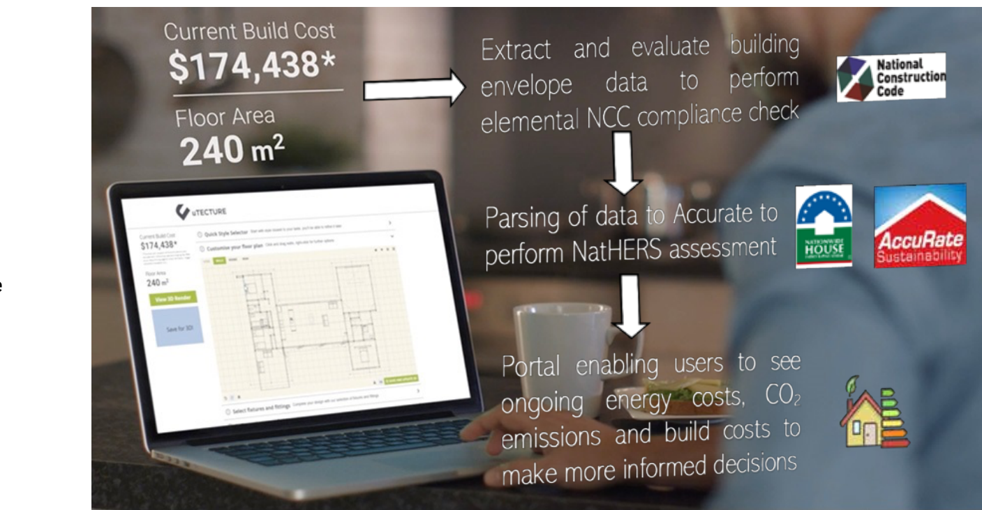
This project developed a comprehensive workflow to take Utexture's existing home design and costing engine and propose subsequent compliance and NatHERS energy rating assessment procedures utilising GSTR's Accurate engine. The developed road map has paved the way for designers, builders, and clients to understand the energy performance and compliance of a home whilst also having an estimate of the capital and ongoing costs in near real time during design.
