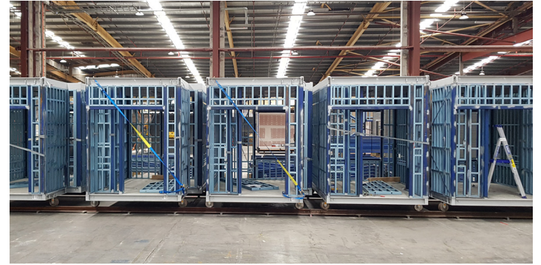
Image credit: Steel framed volumetric module assembly
